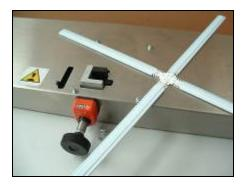
This solution solves the problem of joining Georgian bars and centre keys of different colours or wood-grain finishes. Besides, it is cheaper than to milling system, because it allows to work also thinner Geogian bars (0.4 mm).
